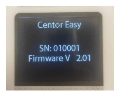
After the self-test, if the unit is functional, the force gauge displays the measurement screen. It then displays 0 N. A tare is performed when the unit starts up.
